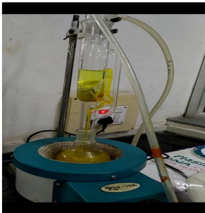
Figure 3: A; Soxhalet unit and B; extracted curcumin
