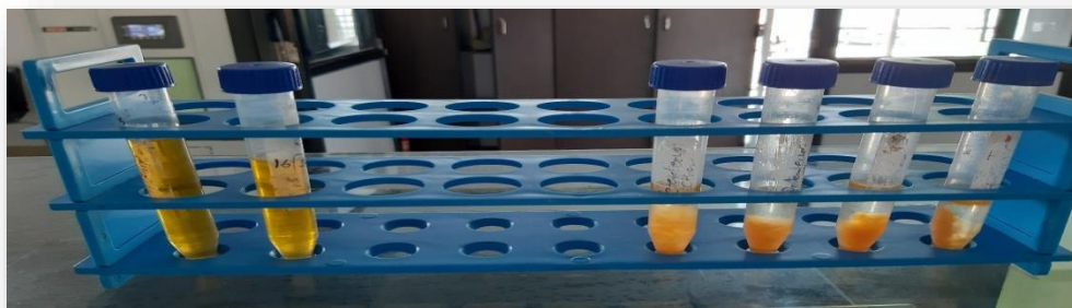
Fig:5. Acetone Petroleum Ether and Hexane Extraction
